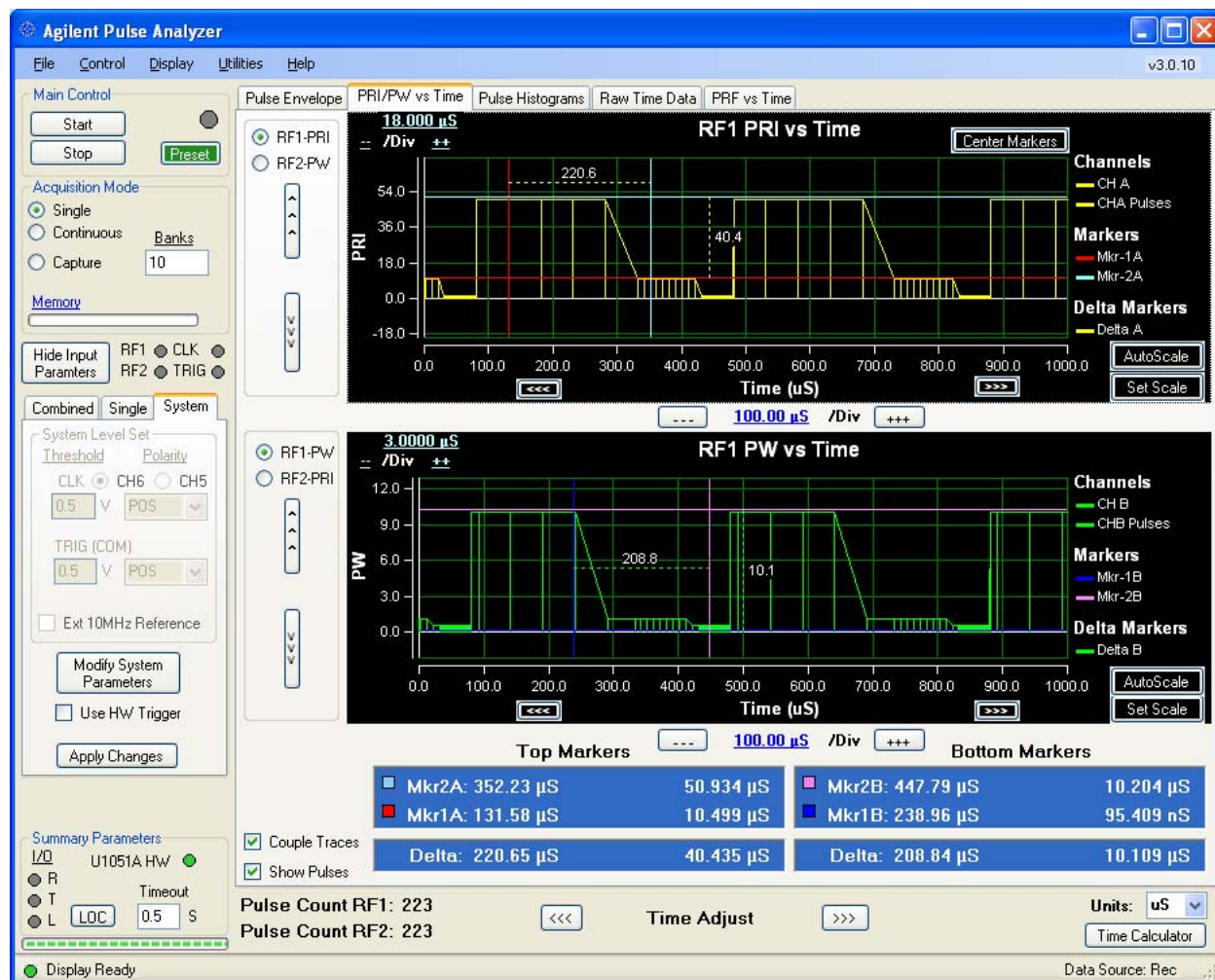
Figure 4.1-8 PRI/PW vs Time 3 Mode Signal
