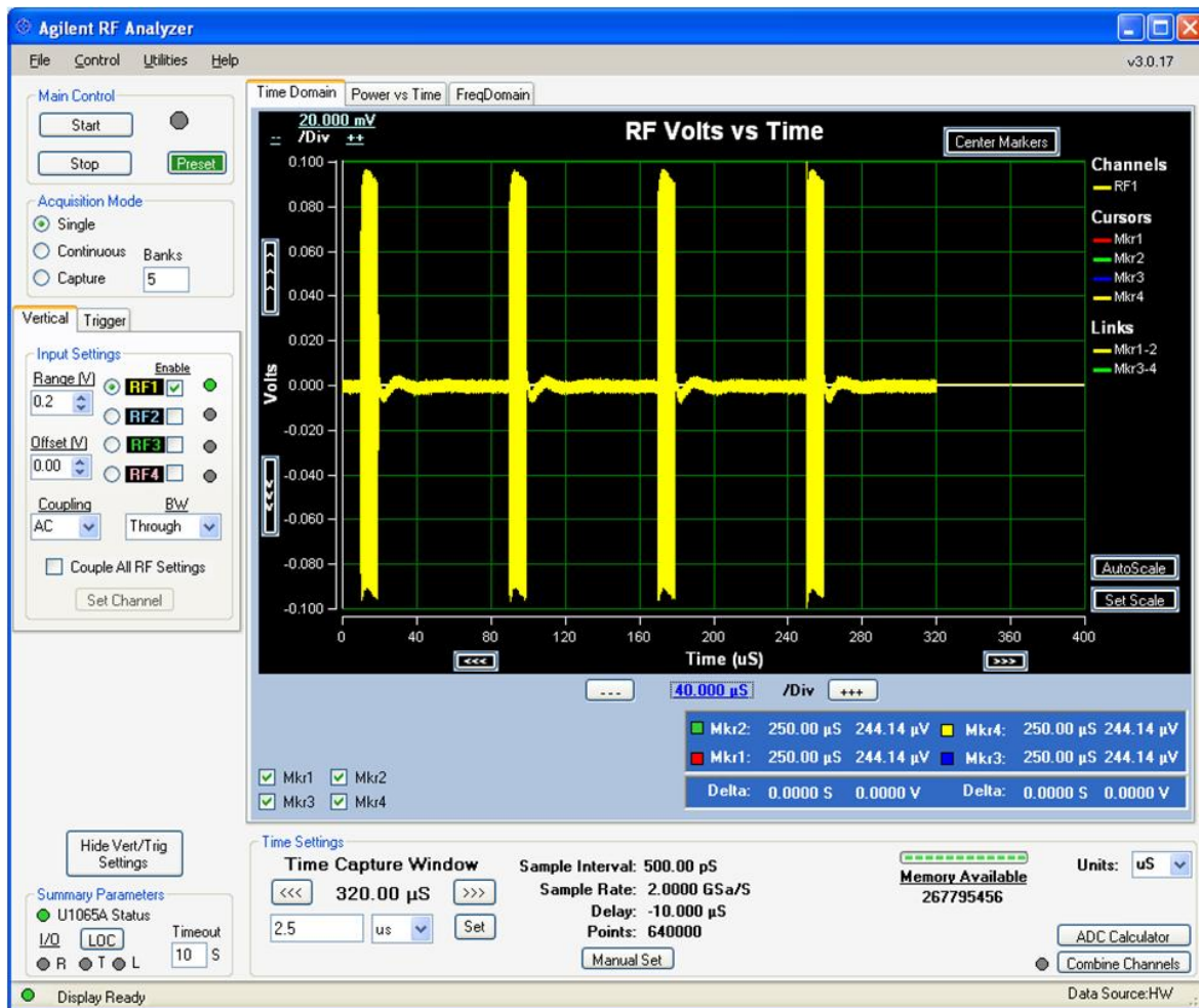
Figure 4.2-2 Pulse Envelope versus Time Display
