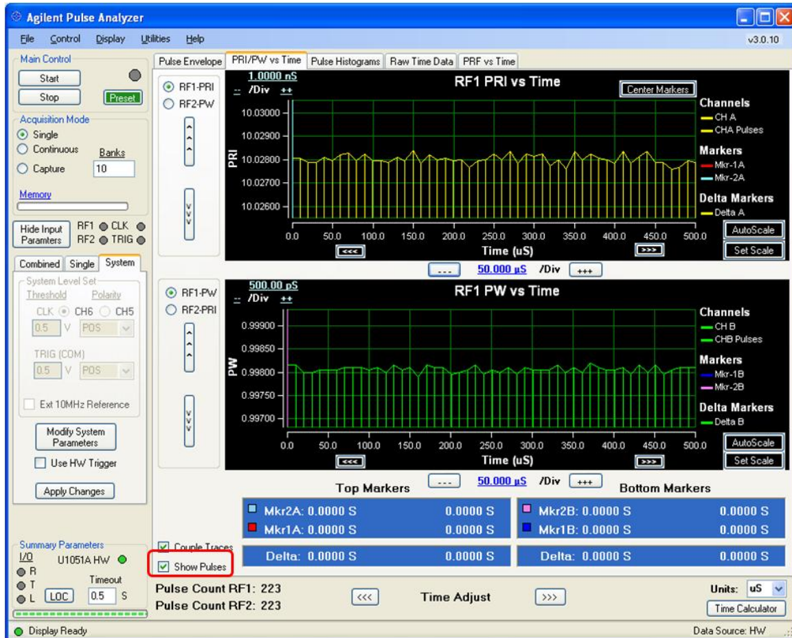
Figure 4.1-7 PRI/PW vs Time with Pulses Shown
