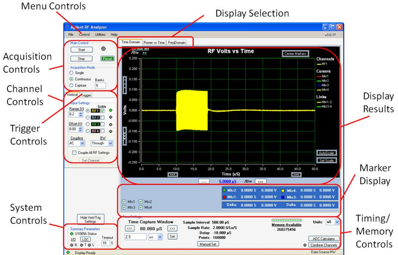
Figure 4.2-1 Agilent RF Pulse Analyzer Software Display
